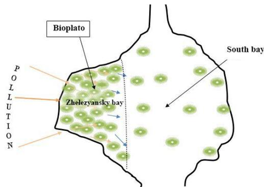
Figure 10: The design of bio plateau to clean the South Bay of the Seversky reservoir.
